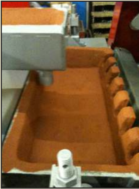
Pouring Bowl - High Quality Refractory Lining
