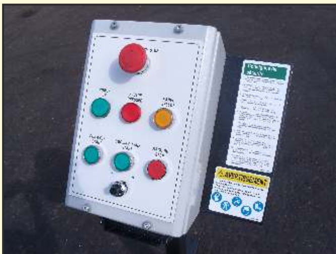
Operator Remote Control Station
