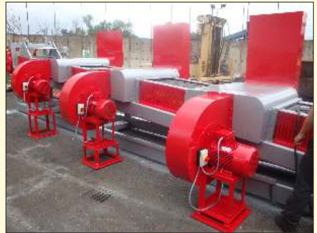
Leviathan Air cooling Fans
